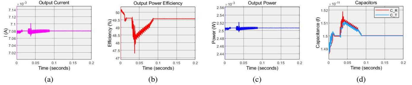
Fig. 9: **Ramp Scenario:** Adaptive Step Controller Performance: a. Output current, b. Efficiency, c. Output power, d. Receiver and transmitter capacitances
