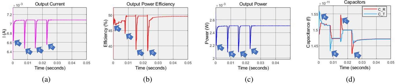
Fig. 7: **Step Scenario:** Adaptive Step Controller Performance: a. Output current, b. Efficiency, c. Output power, d. Receiver and transmitter capacitances
